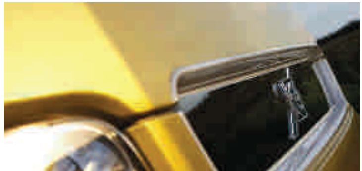
Brøderna Bourghardt manufactures this front part for Volvo buses in TELENE.
