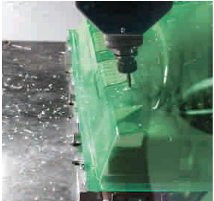
Milling a transparent component in Gibo Plast's Danish factory
