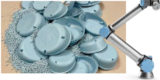
SP Moulding manufactures cover plates for the Cobot series from Universal Robots.
