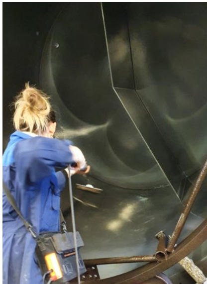
This is a large container coated with Accotron. The thickness of the corrosion coatings is measured evenly across the component
