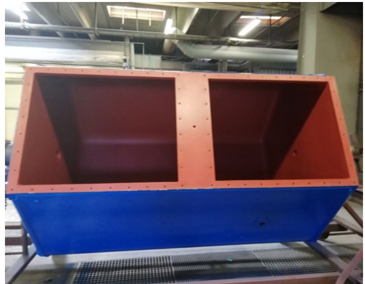
Part coated with Accoshield RF on the inside for non-stick and corrosion protection
